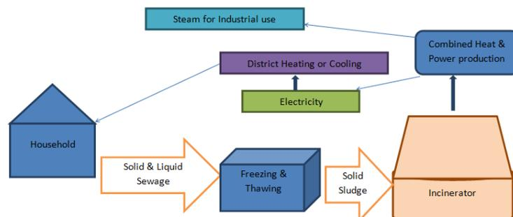
**Figure 3.** Swedish Model II - Incineration after Freezing and Thawing
