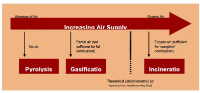
Figure 17. Levels of air (oxygen) present during pyrolysis, gasification and incineration for MSW (Defra, 2013b)
